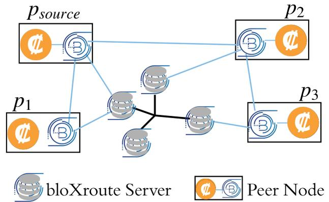
Fig. 1. The components of the *bloXroute* system: the *bloXroute* BDN, and the Peer Network nodes utilizing it. Each Peer Network node runs a Gateway process as an intermediary between its blockchain application and the *bloXroute* BDN.
